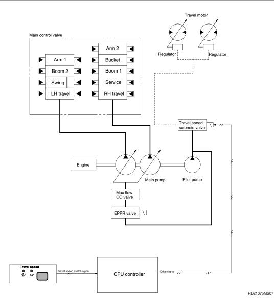
Travel speed can be switched manually by pressing the travel speed switch on the cluster.
